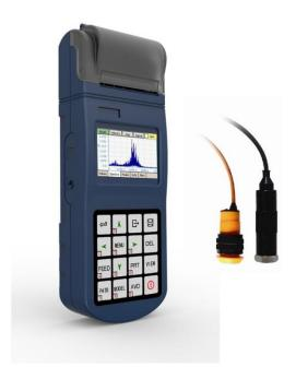
PV400 uses piezoelectric acceleration transducer to convert vibration signal into electric signal. Then by analyzing input signal, results including RMS of velocity values, peak-peak value of displacement, peak values of acceleration or real-time spectral charts are displayed or printed out. It can not only measure the three parameters, but also for rotational speed measuring.
